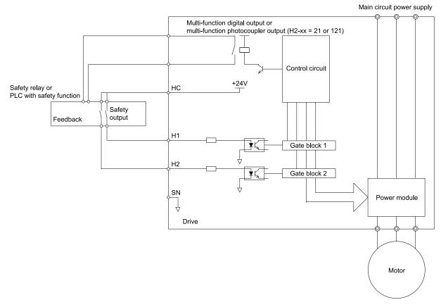
Figure 3.2 Safe Disable Function Wiring Example
