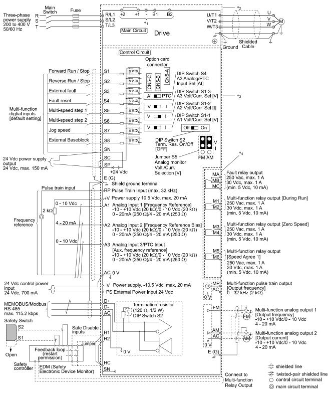
Figure 1.2 Wiring Diagram for Low Voltage Directive Compliance
