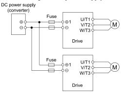
Figure 1.3 Wiring Example for DC Power Input
